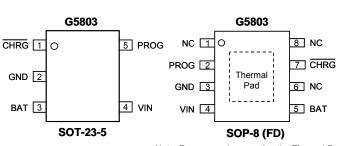
Note: Recommend connecting the Thermal Pad to the Ground for excellent power dissipation.
