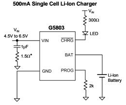
\*1.5Ω resistor in series with a ceramic capacitor will minimize the start-up voltage overshoot transients
